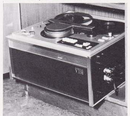
HIDDEN RECORDER makes a continuous 7-hour videotape of all comings and goings in the banking chamber — including hold-ups.
