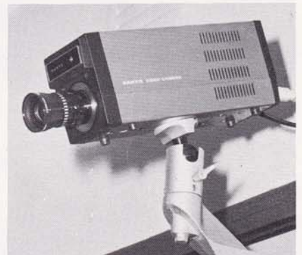
TV CAMERA, with wide-angle lens trained on counters, operates continuously all day from inaccessible position on back wall of office.
